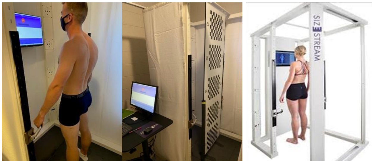
Figure 2. SizeStream SS20 Three-Dimensional (3D) Circumference Scanner. (left) active scanning of a volunteer; (center) scanner setup at one of the study locations; (right) image from the company.
